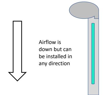
UV-C Chamber Side View as Mounted to the wall.
